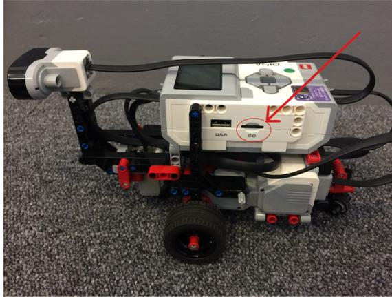
Figure 2.3: The SD slot on the EV3 brick
